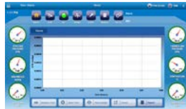
The Home screen shows the Carrier and Test Gas pressures, barometer, and block temperature.
